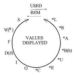
The values displayed can be adjusted with the ADD/FULL toggle switch. ADD increments the value, and FULL decrements the value. As you hold ADD or FULL, the scrolling rate will increase up to a maximum speed.
