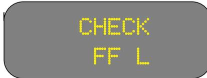
"CHECK FF L" indicates a bad fuel flow input channel for the left engine. Other possible error messages are listed below:
