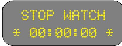
Press START/STOP switch to operate the stopwatch. The RESET button resets the timer. Use the PAGE/UP DOWN or rotary switch to return to the main display functions.
