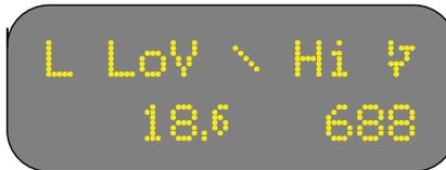
Note that the "-" symbol has changed to a "\". This indicates that the engine is performing the start up.
