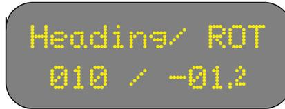
In the above example, the aircraft is heading 10 degrees, and is turning left at 1.2 degrees per second.
