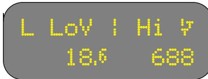
The "\" symbol has now changed to a "!" symbol indicating the engine has completed the start up procedure, and is now running.
