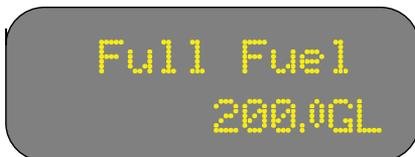
Entering the full fuel amount is only necessary during the initial setup. The ETM stores this value in its memory, permanently.
