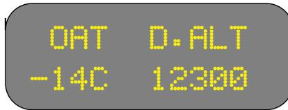
■ A typical OAT and static air temperature (SAT) display looks like this:
