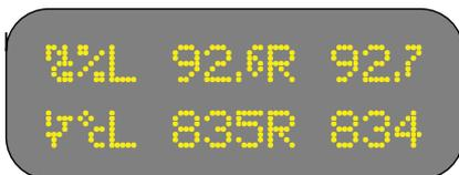
**2. Torque (TQ) and Turbine Temperature (ITT or TOT)**
