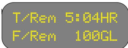
In the above example, the aircraft has about five hours of flight time, and one hundred gallons of fuel remaining.
